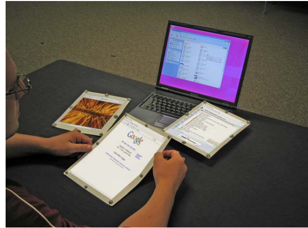
Figure 2. PaperWindows prototype with three pages.
