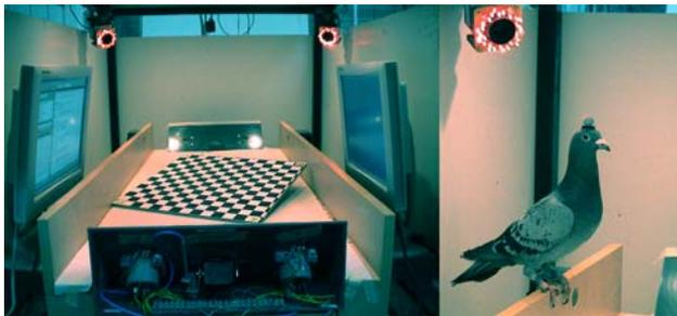
**Fig. 2** Setup of the motion capture system during calibration (*left*) and placement of the marker on the pigeon's head (*right*)
